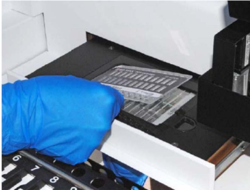
Figure 2: Load PCR Cartridges
