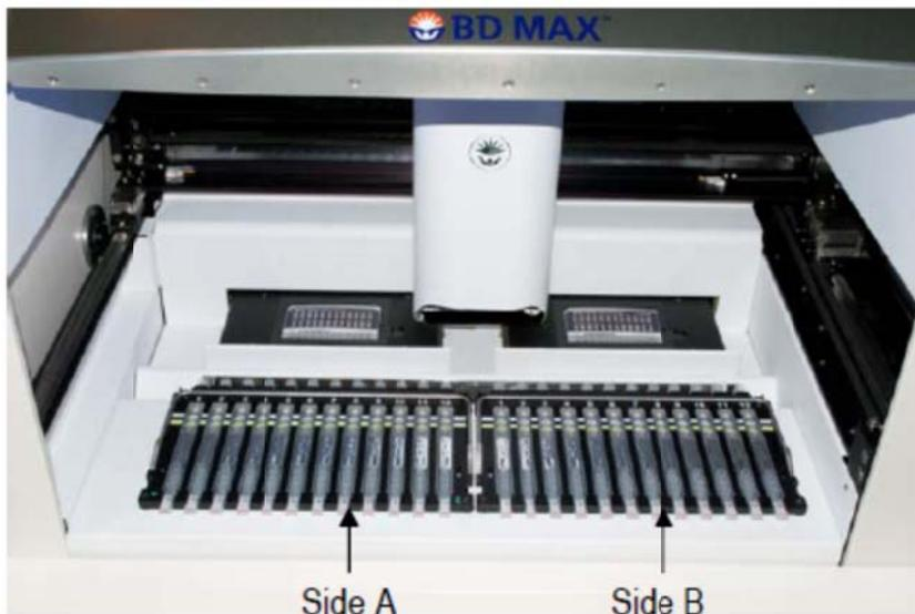
Figure 3: Load Rack(s) into the BD MAX™ System.
