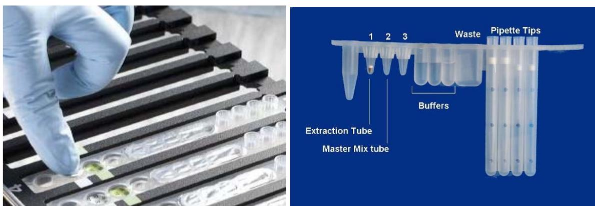
Figure 1: Snap BD MAX™ StaphSR Extraction tubes and Master Mix tubes into reagent strip
