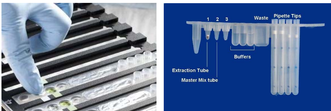
Figure 1: Snap BD MAX™ MRSA XT Extraction tubes and Master Mix tubes into reagent strip
