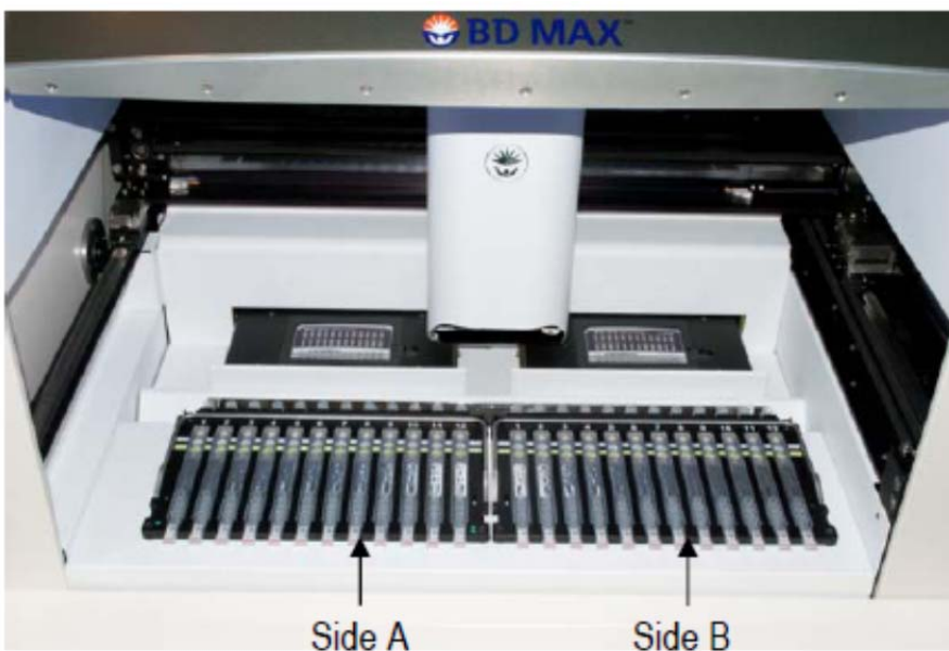
Figure 3: Load Rack(s) into the BD MAX™ System.
